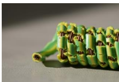
Pic 3 Cable insulation degradation caused by thermal aging
