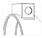
• Terminal boxes are excellent for preventing electrical shock or electrical shorts. Terminals boxes are available on any clamping or construction style.
