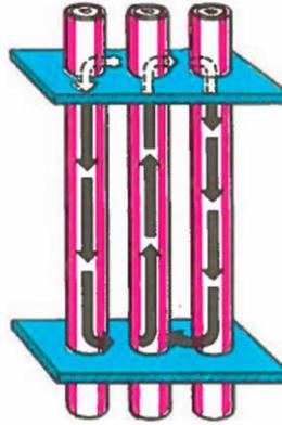
On a 50 cycle supply the losses from eddy currents are very small and can be ignored. In the case of circulating currents these also may be unimportant but the following points should be borne in mind.
