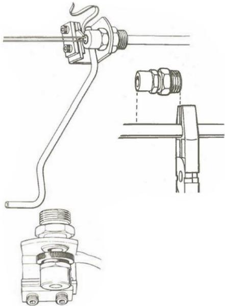
Just clears the thickness of the sheath without fouling the conductors; it should protrude just beyond the half-way mark, which can be pencilled on the gland (B). Ensure blade is in pressure contact with gland (C) and tighten holding down bolts. Insert cable end into gland, apply pressure and rotate tool in clockwise direction so that the blade engages the sheath. Spare cutting blades are obtainable from any MICC Branch Office.
