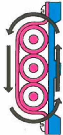
When running large single conductor cables they should not be spaced apart but should be in trefoil formation or certainly in very close proximity to one another. Circulation of air around the cables will obviously be beneficial and this can be improved by the use of standoff or spacer bar saddles, as shown above.
