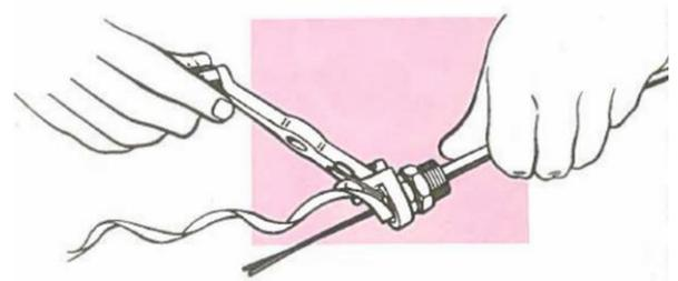
**Method 4 - Using rotary stripping tool**
