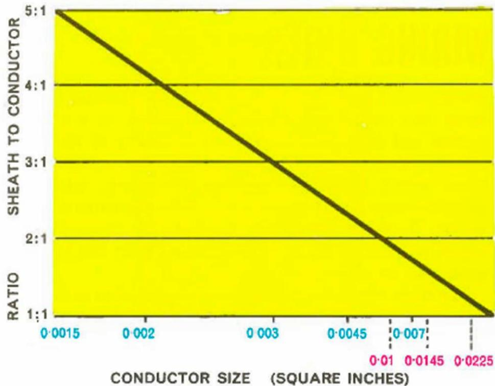
Multi-conductor cables can, however, be used no matter what their size, since in all cases their sheaths are more conductive than any one conductor.
