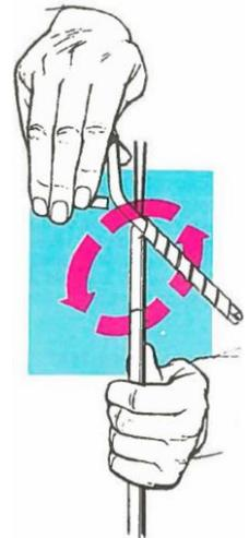
**Method 3 - Using rotary stripper / pot wrench tool**
