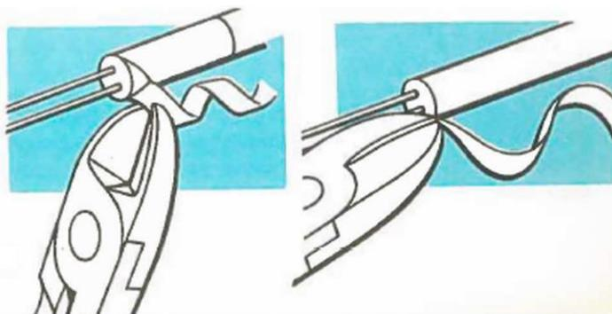
**Method 2 - Using fork-ended sheath stripper**
