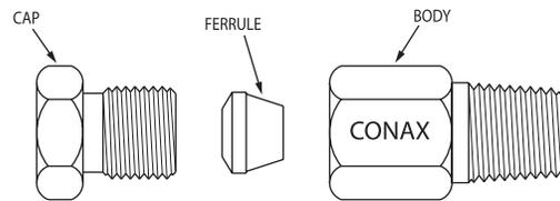
Glands are supplied factory lubricated. If glands are cleaned prior to assembly or when reused, the glands should be relubricated to maintain the published torque and pressure ratings. See page 103 for information on our lubrication kit.
