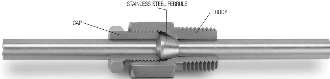
Conax Technologies Model MK Midlock Glands seal a single tube or probe. Featuring a metal-to-metal seal rather than our standard soft sealant technology, MK glands are used where a joint must be opened and resealed in the same setting. Their unique design forms the seal well within the body housing to provide superior performance in high vibration applications.
